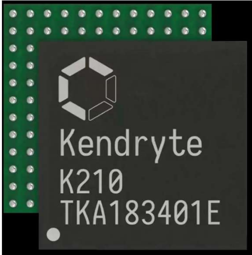
Kendryte K210 MCU Package: Ball Grid Array (BGA) 19
